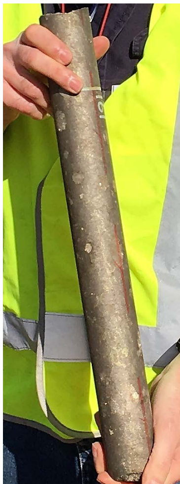
Figure 4 – drill core from MAD60 with large pentlandite crystals prominent in the core. This section of core is from an interval that returned assays of 3m @ 6.40%Ni, 3.55%Cu, 0.21%Co and 5.25g/t total PGEs from 159.38m.
