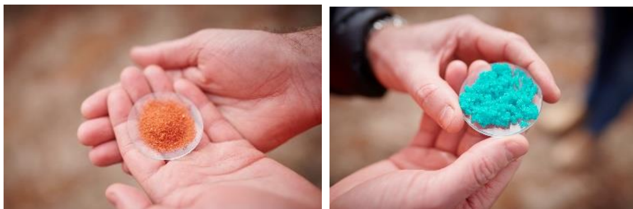
Figure 3: Samples of cobalt sulphate (left) and nickel sulphate (right) produced from Clean TeQ Sunrise
