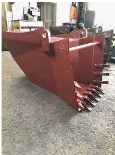
The ground engaging tools in the buckets are also subject to high wear rates
