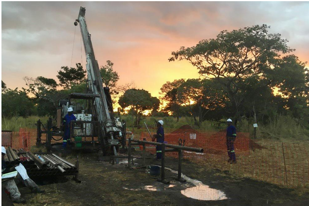
Figure 1. Diamond Drilling during Mustang’s Scoping Study Drilling Campaign
