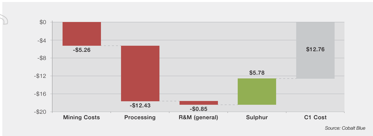
Figure 7. Thackaringa Cobalt Project – Production Target – C1 Site Cash Cost US$/lb (net of by product)
