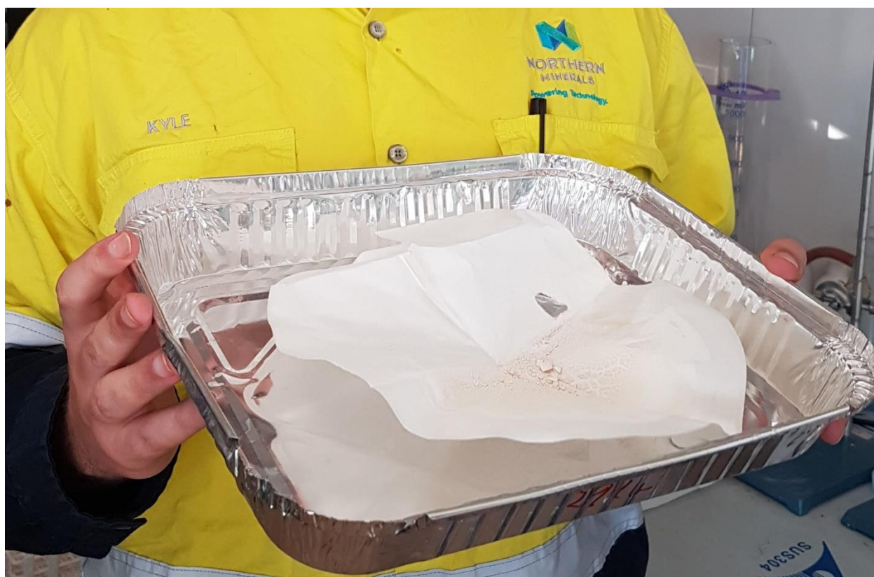
Rare earth carbonate from on-site laboratory
