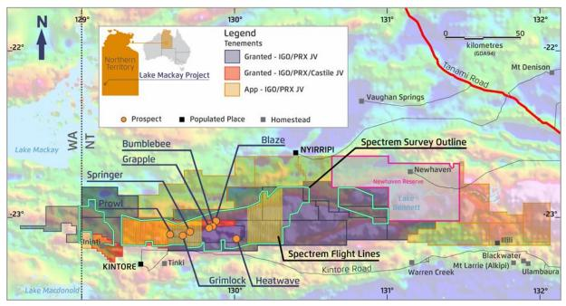
Figure 3. Lake Mackay JV area highlighting active prospects and Spectrem AEM survey lines completed (orange) and planned survey area (blue outline).
