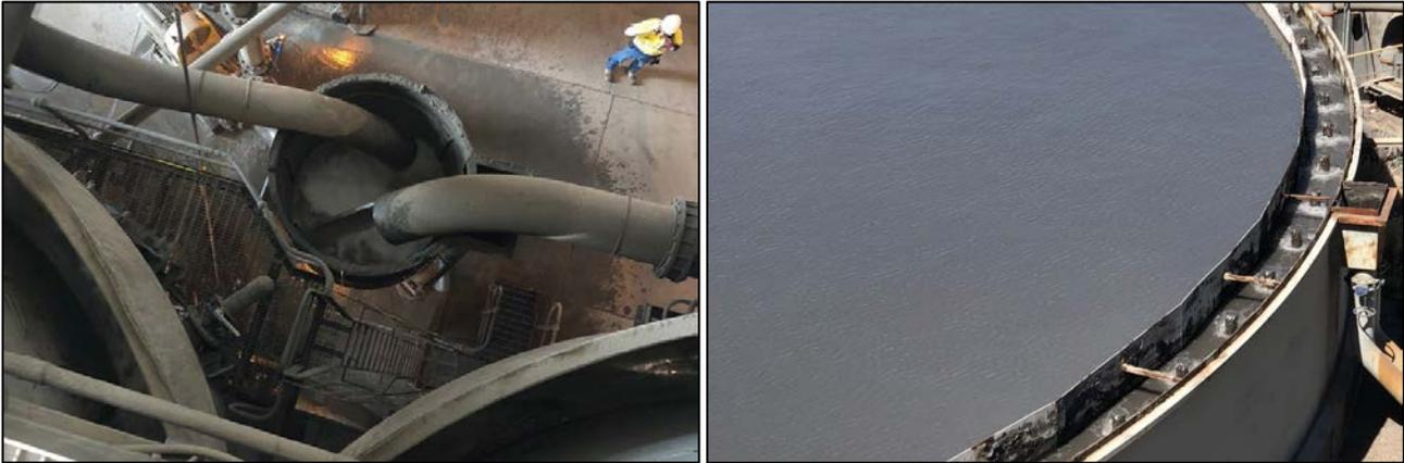
Figures 8 & 9: Water exiting the final conc. float cells (left) & zinc thickener commissioned for operations (right)
