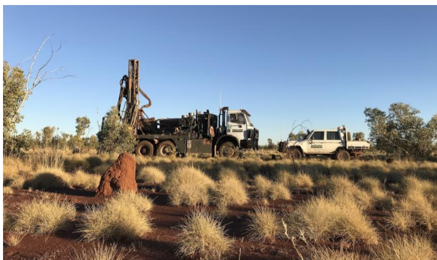
Figure 2. Aircore drilling underway at the Capstan Prospect
