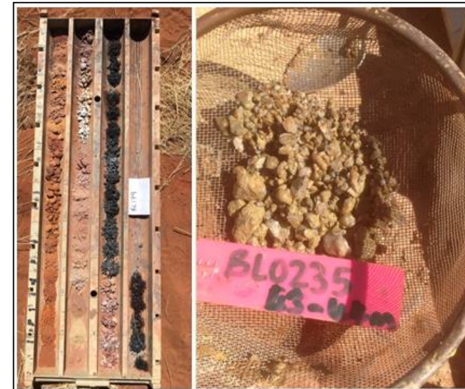
Black shale and sulphide with veining in saprolite intersected in aircore drilling
