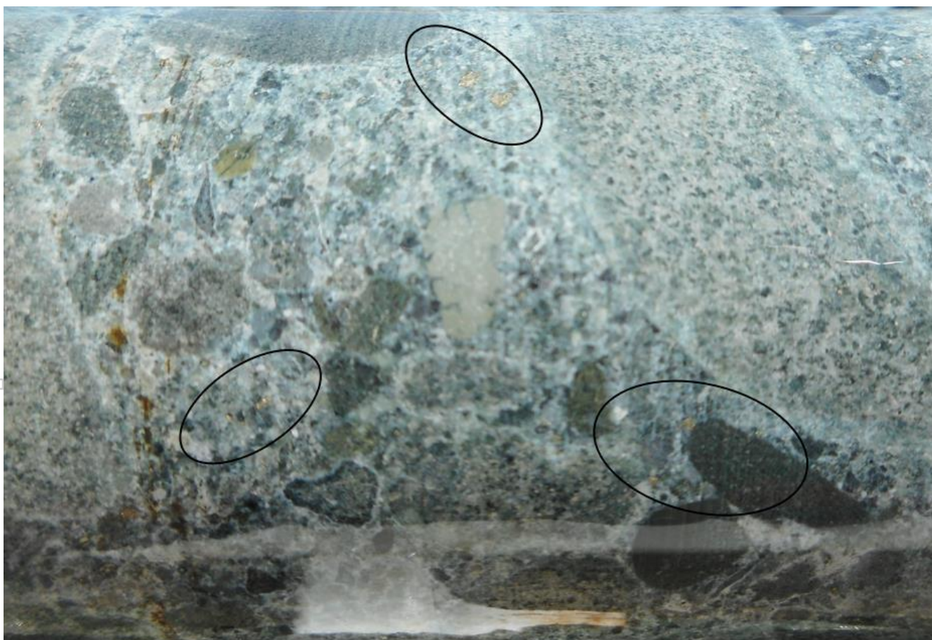
Plate 4 Detrital pyrite in sericite-chlorite alter pebble to cobble conglomerate at 46.90m (core diameter 61.10mm).
