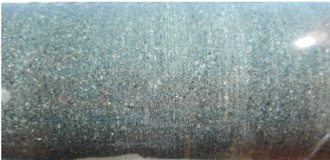
Plate 4 Detrital pyrite in sericite-chlorite alter pebble to cobble conglomerate at 46.90m (core diameter 61.10mm).
