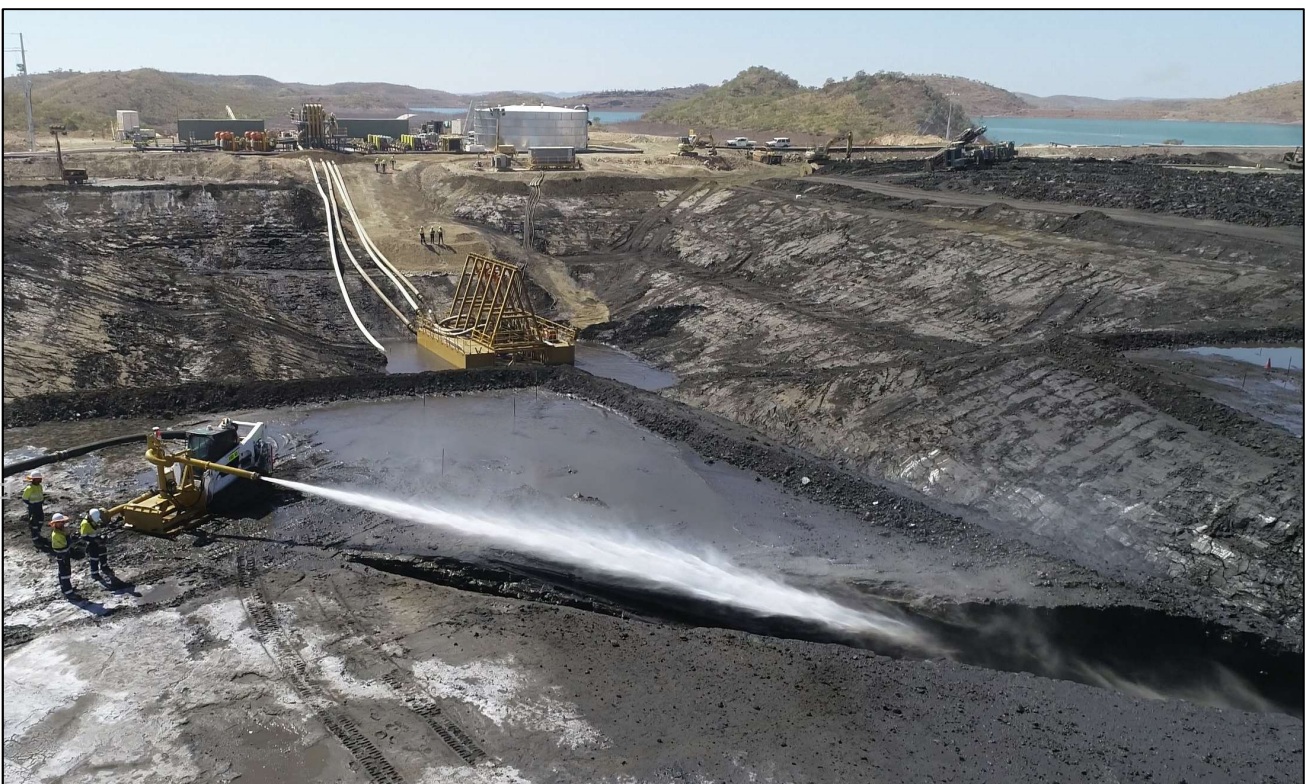
Figure 2: Hydraulic mining of tailings into the Slurry Winning Pontoon at the Century Tailings Deposit
