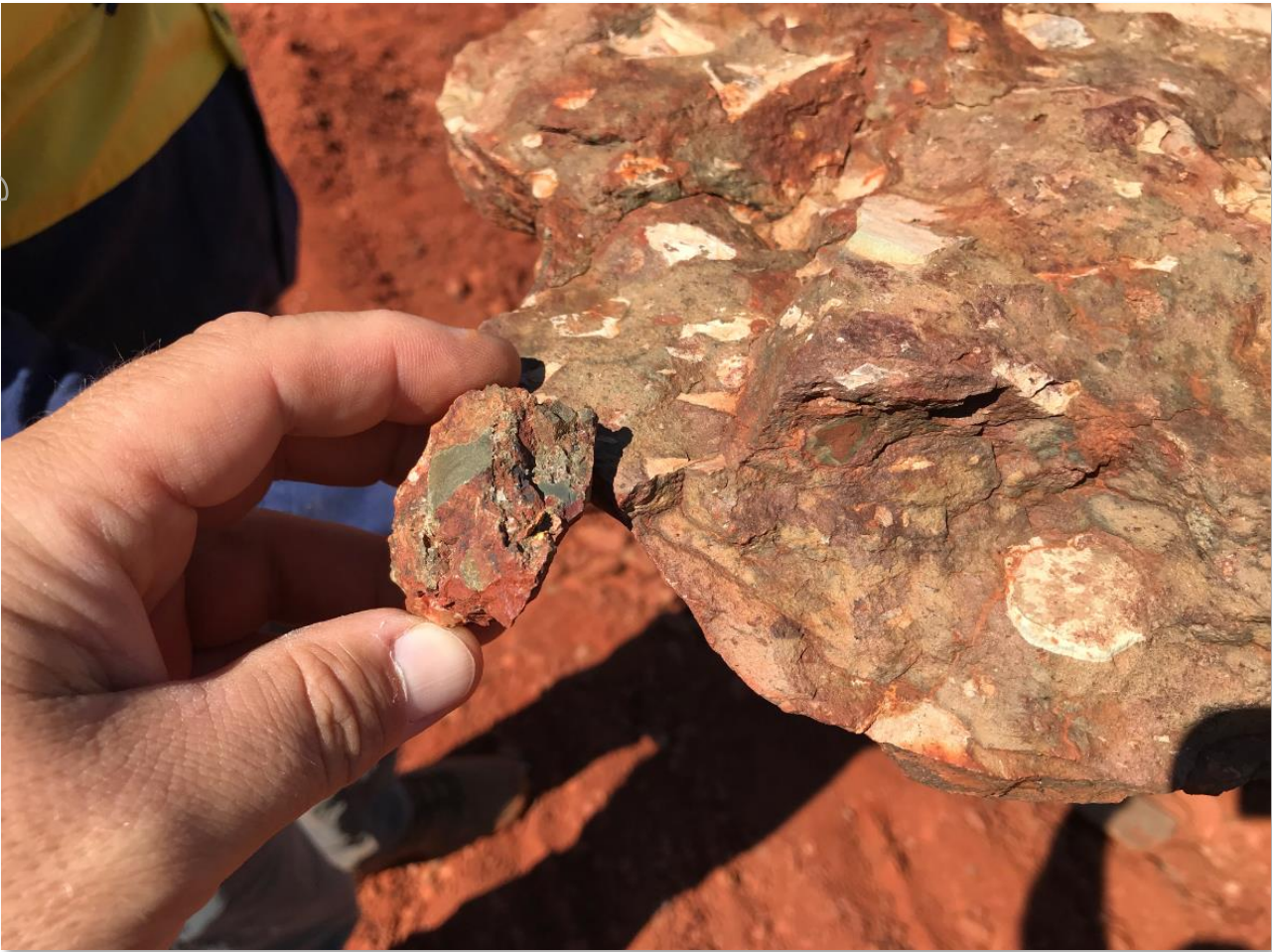
(Figure 2 – Piece of conglomerate from Purdy’s Reward (left) displaying fragments of mafic tuff. Note the gold nugget embedded in matrix. A sample of mafic tuff from the marker unit at Comet Well (right).
