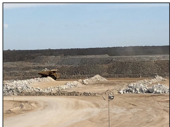
Run of Mine stockpile fingers
