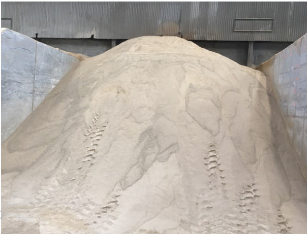
CAPTION: Run of mine Ardmore phosphate rock ore at customer bunker ready for large-scale SSP plant trial.
