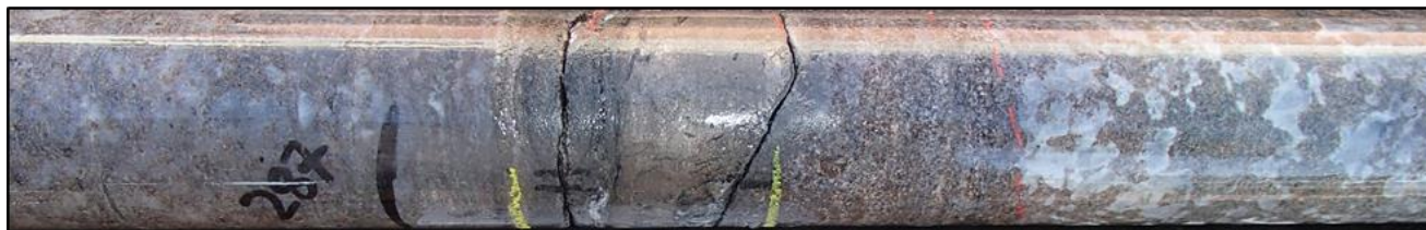
Figure A-2: Typical sulphide mineralisation from drill hole OROD001 showing the injected semi-massive and stringer sulphide, very coarse blebby sulphide and infiltration sulphide. The percentage of sulphide in a sample interval rarely exceeds 5%, but the high tenor zones are enriched in base and precious metals.
