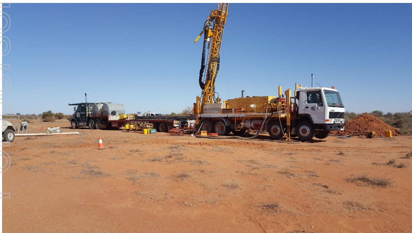
Figure 1: Diamond drilling in progress at Kalkaroo to obtain large diameter PQ core samples for metallurgical test work.
