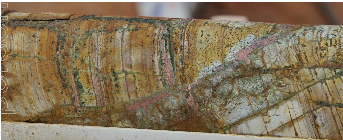
Figure 5: Seams of native copper (copper metal) representing secondary, supergene copper mineralisation hosted by weathered and oxidised bedrock (saprolite).
