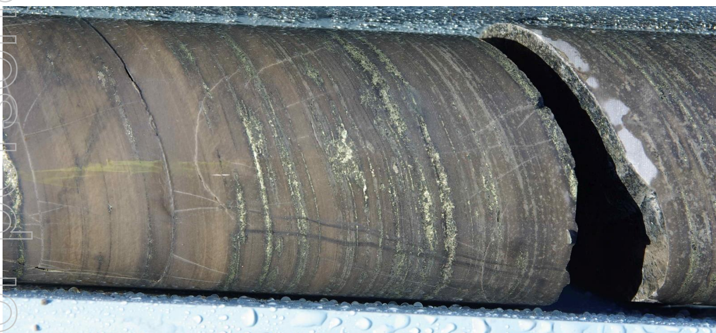
Figure 7: Bedding replacement chalcopyrite (copper sulphide) and pyrite (iron sulphide) mineralisation representing primary sulphide mineralisation in fresh host rock.
