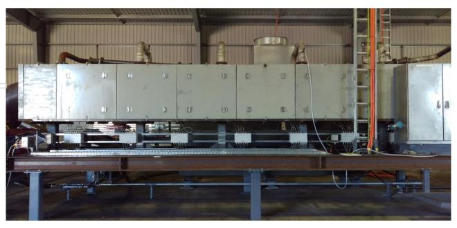
Fig 3 - Part of the Thermal Desorption Unit
