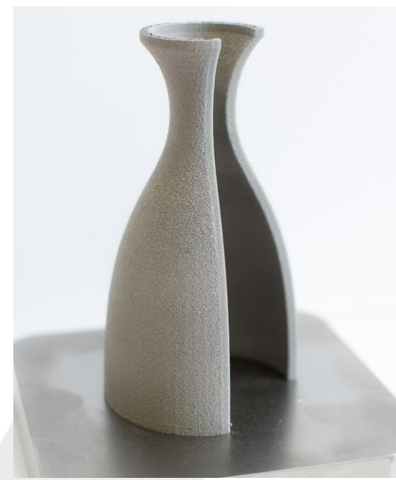
Complex de Laval Rocket Motor Nozzle Cross Section printed with Alpha RMT printer
