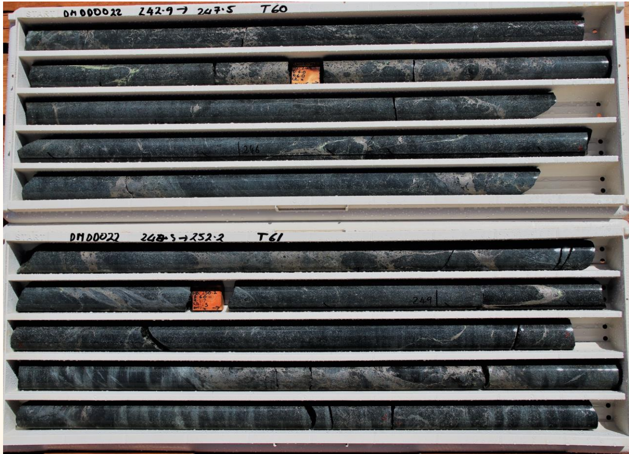
Figure 2. Well-developed 10 metre mineralised interval displaying strong disseminated and moderate net textures and lesser massive sulphide mineralisation from DMDD0022, core is NQ, from 242.9-252.2m downhole.
