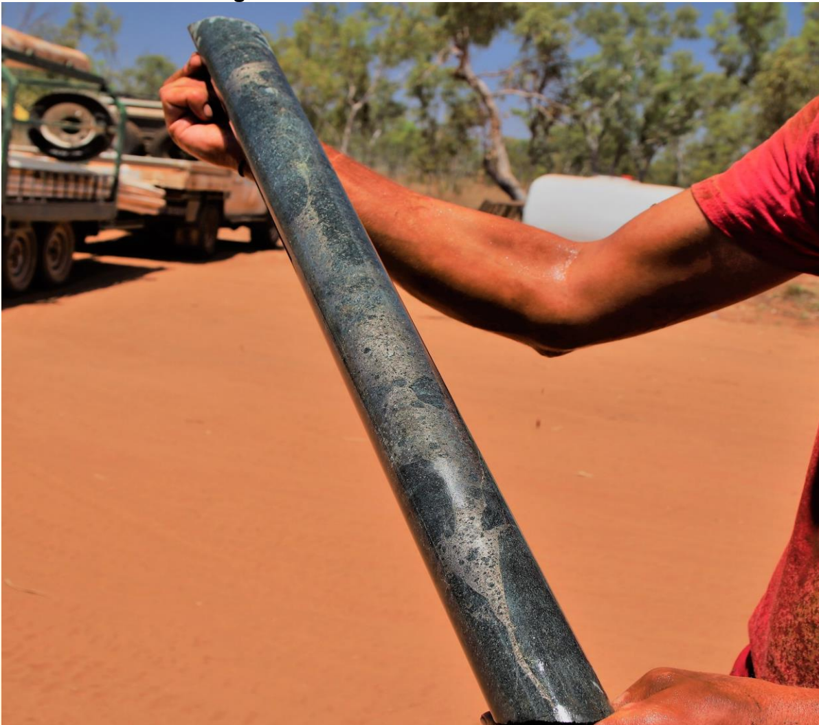
Figure 1. Well-developed sulphide mineralisation from DMDD0022 with visible Pentlandite, Chalcopyrite & Pyrrhotite; photograph is of NQ whole core, 247.5.-248.10m downhole.
