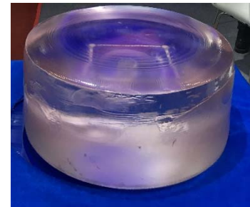
20 inch Sapphire boule to be cut and polished for space research lens
