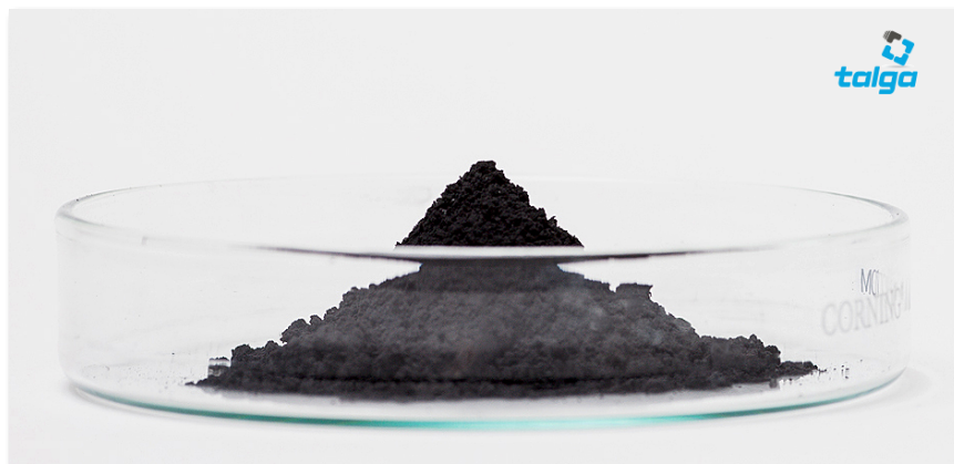
Figure 1 Talga's Li-ion anode product ready for aqueous formulation and coating onto current collector.
