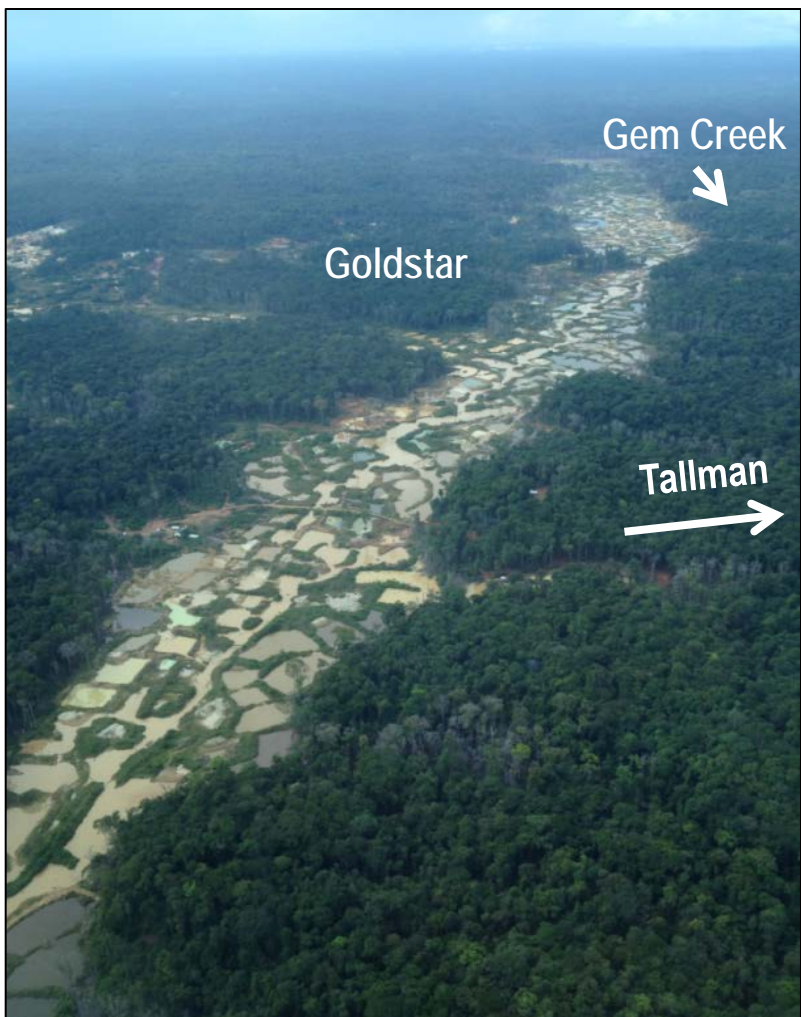
Aerial photograph showing extensive alluvial workings
