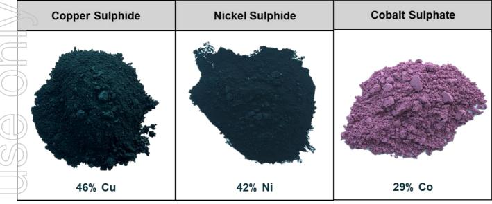
Copper, nickel and cobalt products produced in the Mt Venn Metallurgical Testwork
