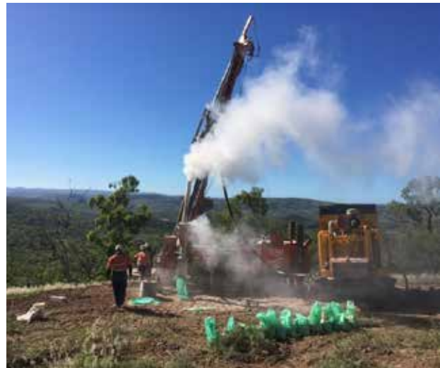
Figure 7 Reverse circulation drilling at Bunyip.
