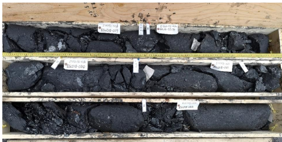
Field Photos of 150mm Diameter Coal Core Samples from the First Borehole
