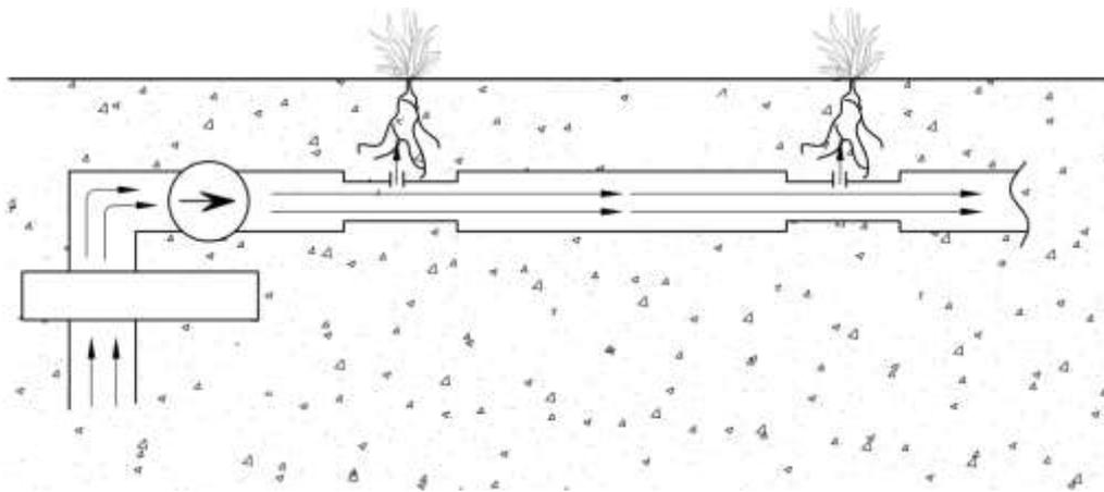
*Roots’ patented ‘smart pipe’ system provides targeted heat and cooling delivery to plant roots at increased energy efficiency due to insulation of the pipe between the plants*
