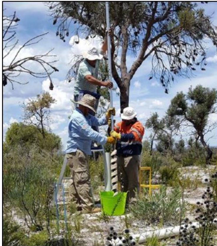
Figure 7: Sand sampling using a hand auger at Muchea
