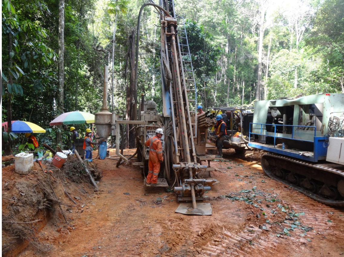
Schramm RC drill rig with Compressor and booster on TRC001
