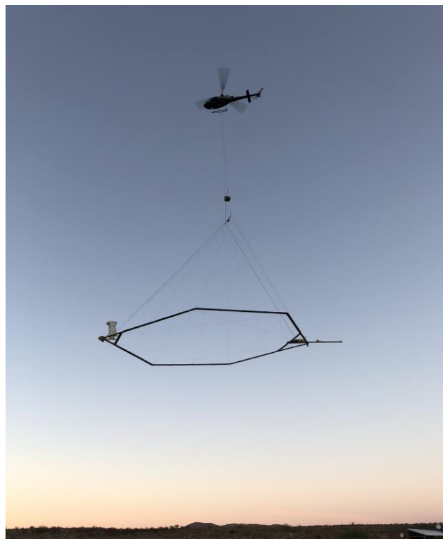
Figure 3: The SkyTEM™ technology during survey operation (during the 2017 – 2018 regional survey).
