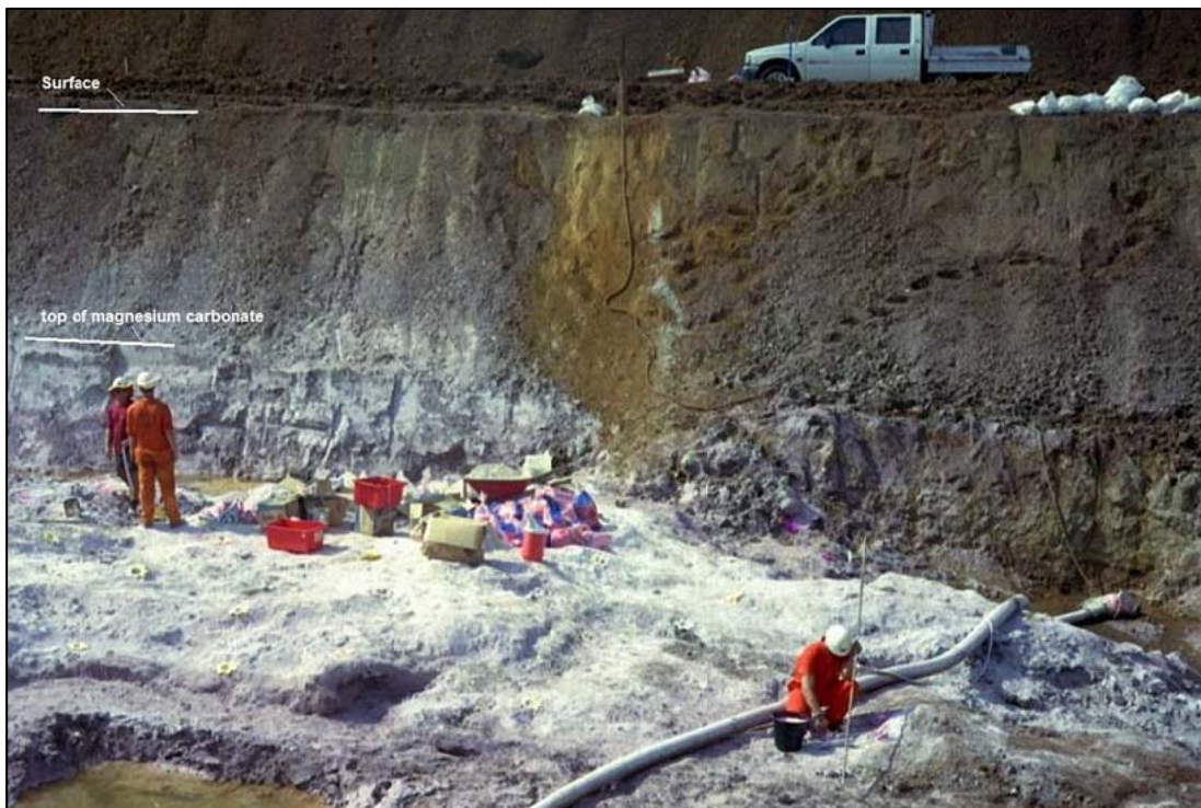
Figure 4 Test mining of magnesium carbonate at Winchester (setting of charges)
