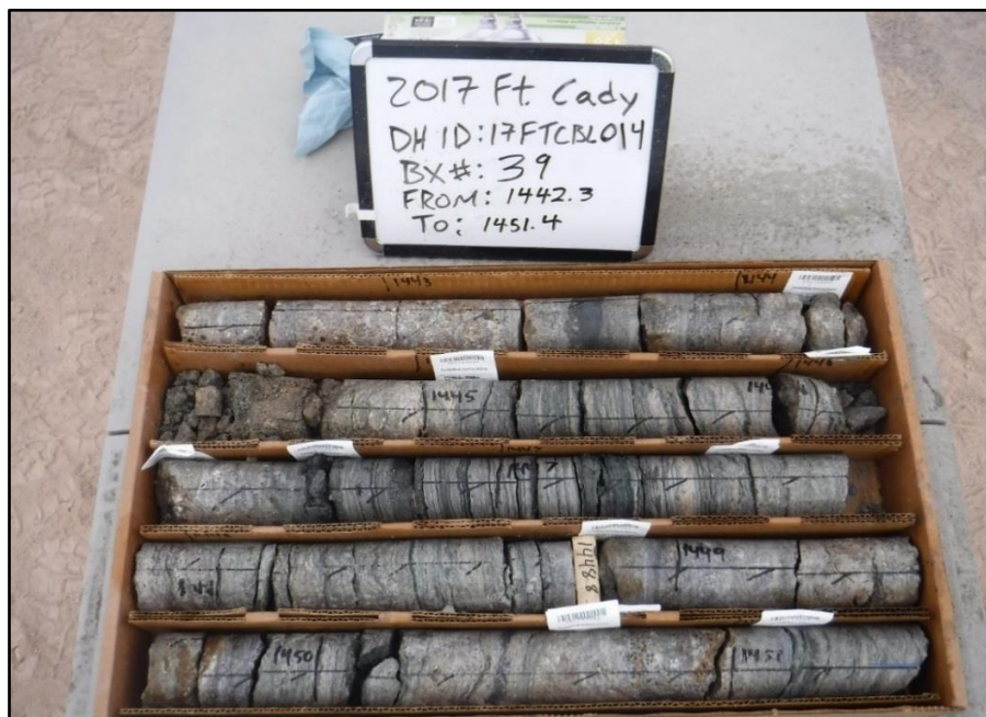
Figure 12. Core photo, 17FTCBL-0014, Note the variability of the core, including finely banded clay, and more competent evaporitic (mostly anhydrite, the lightest coloured material) sections. Depth measurements are in feet.
