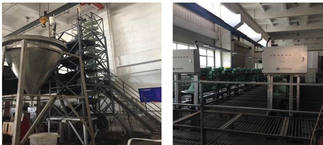
Figure 11: Hunan Research Facility spiral and flotation circuits
