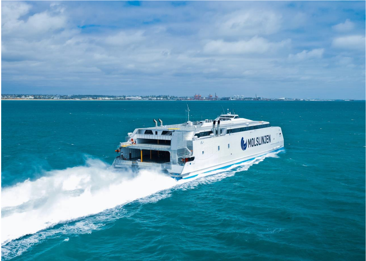
Express 4 (Hull 393) is the largest (by volume) ferry designed and constructed by Austal and is capable of transporting over 1,000 passengers and 425 cars. (Photo Credit: William Blaauw)
