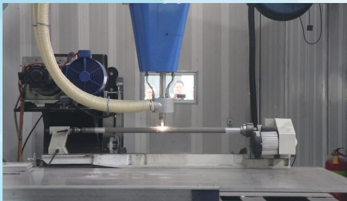
Titomic Kinetic Fusion™ demonstrates mandrel deposition at Titomic R&D Production Centre in Melbourne yesterday.
