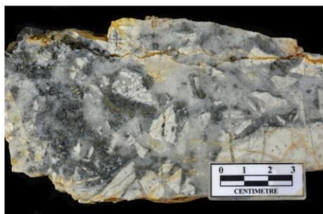
Photo A: Sample KRS205254. Hydraulic vein breccia, with angular rhyolite clasts, set in a flood mesocrystalline silica-sulfide matrix (pyrite, chalcopyrite, silver sulfosalts). 13.3 g/t Au and 2,130 g/t Ag.
