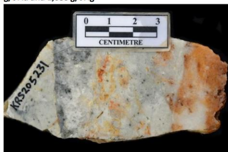
Photo B: Sample KRS205231. Hydraulic vein breccia, comprised of white silica-illite/adularia altered rhyolite fragments engulfed by mesocrystalline to crystalline quartz with coarse-grained sulfides (pyrite, tetrahedrite & silver sulfosalts). 9.23 g/t Au and 1,080 g/t Ag
