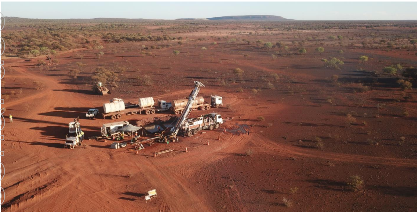
Plate 1 - Diamond drill rig on site at the Gabanintha Project
