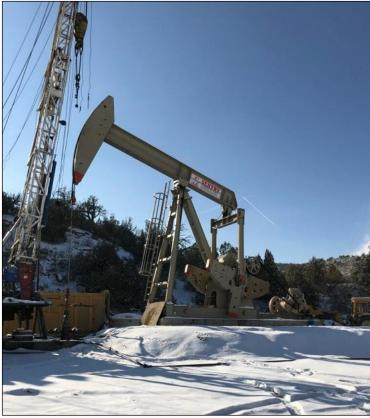
Figure 1: Pump jack installed on the JW #23-25 Well
