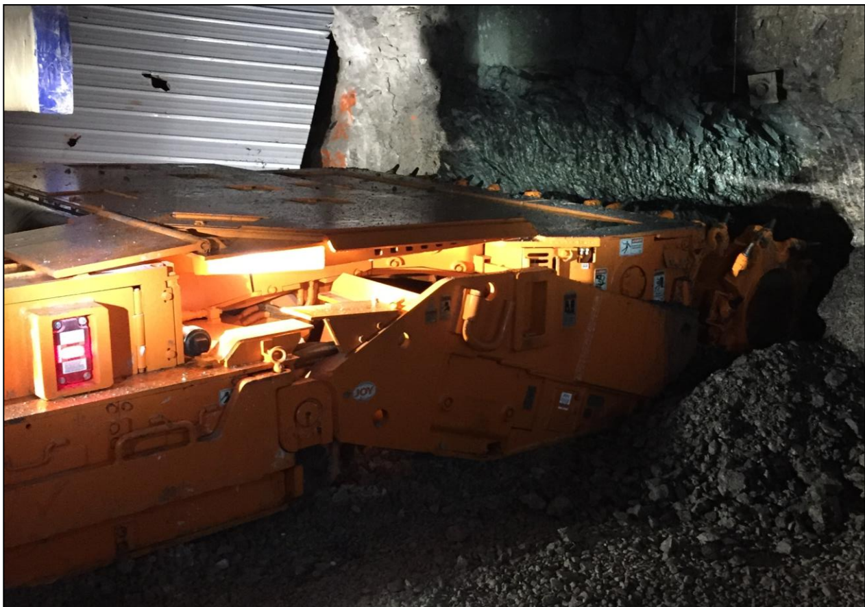
Figure 2: Paringa's continuous miner cutting coal at the Poplar Gove Mine
