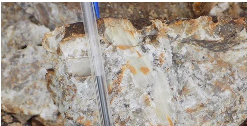
Figure 4: Rock Chip Sample collected showing white spodumene (the large, long prism to right of the blue pen) in a quartz feldspar matrix
