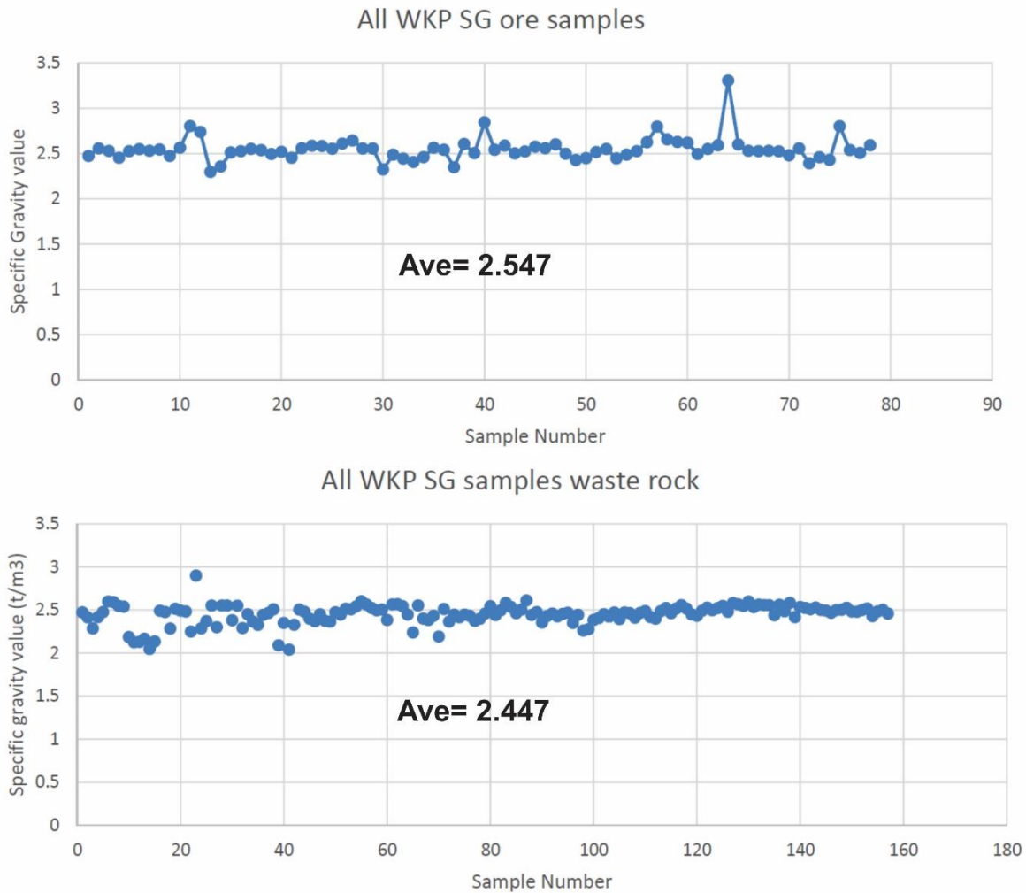
Figure 11.2 Charts showing the SG values calculated for ore and waste rock samples at WKP
