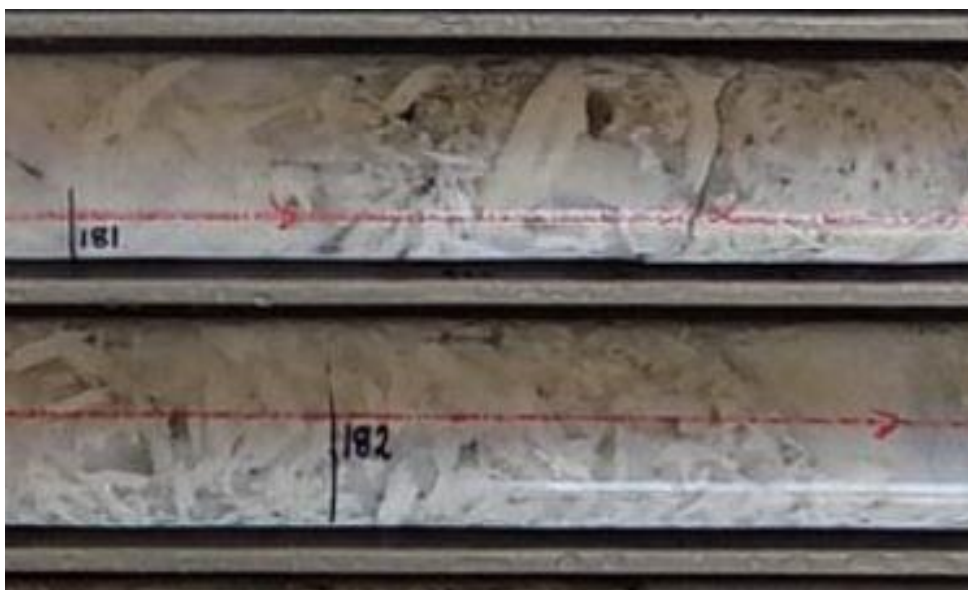
Figure 3: Close up of core from 181 to 182 metres in drill hole CD18DD006 with very coarse spodumene throughout the interval
