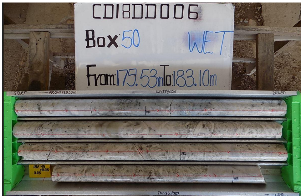
Figure 2: CD18DD006. 181 – 182m 4.65% contained \text{Li}_2\text{O}
