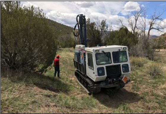
Figures 3 & 4: The Track Drill machine (L) and a Buggy Drill machine (R) undertaking the 3D seismic program
