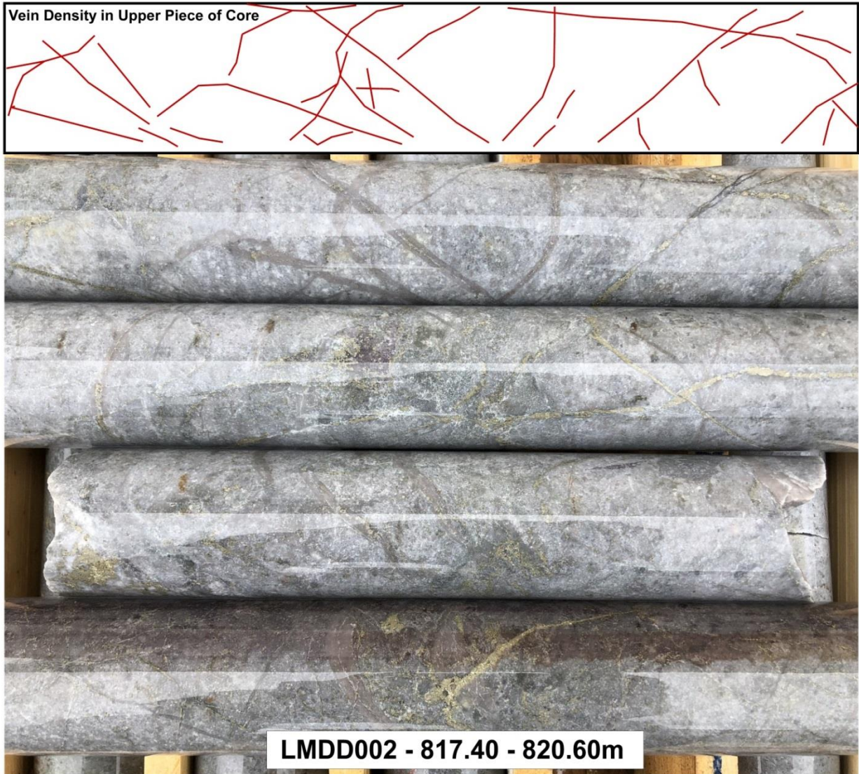
Plate 5 – Developing quartz B-vein stockwork and late-stage pyritic D-veins in phyllic-altered protolith in LMDD002, and illustration of fracture density.
