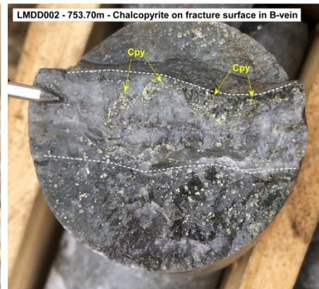
Plates 6 and 7– Molybdenite and chalcopyrite smears and disseminations on some fracture surfaces in LMDD002.
