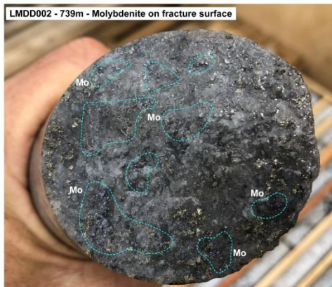
Plates 6 and 7– Molybdenite and chalcopyrite smears and disseminations on some fracture surfaces in LMDD002.
