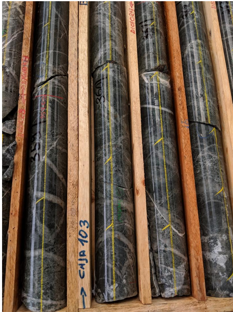
Plate 1: Example of intense porphyry-related quartz stockwork veining in diorite within drill hole BMDD001 (358.70 – 362.00m) downhole at Bramaderos Main.
