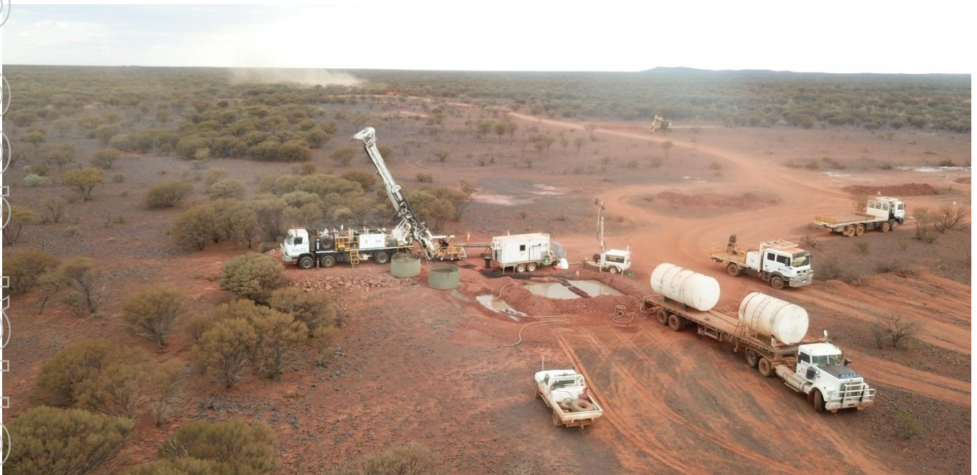
Figure 3 Diamond drill rig on site at the Australian Vanadium Project
