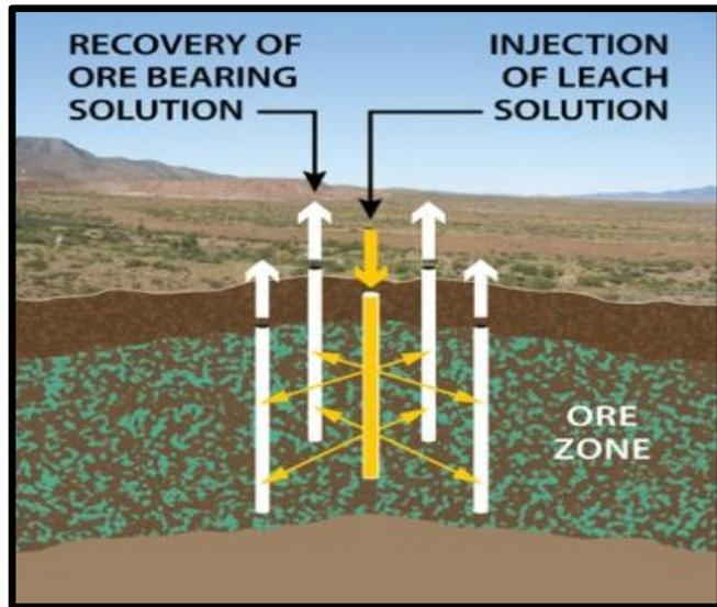
Figure 2. Schematic of In Situ Recovery process
