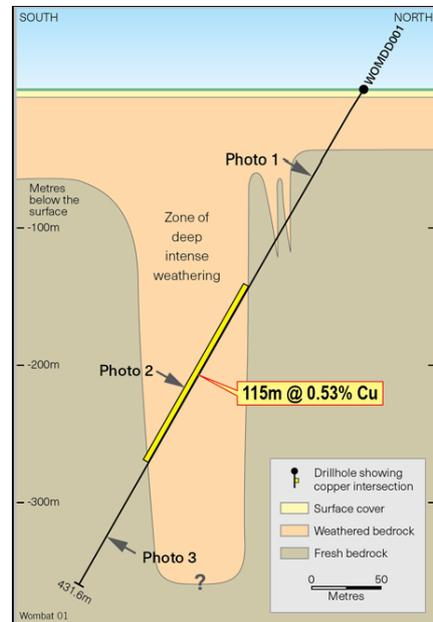
Figure 4 - Wombat section showing weathering trough
