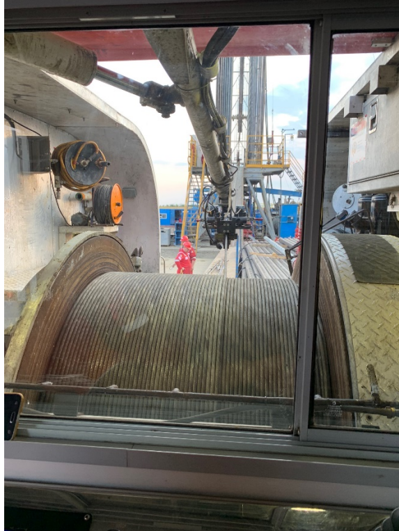
Electric line logging in 8 1/2" hole
