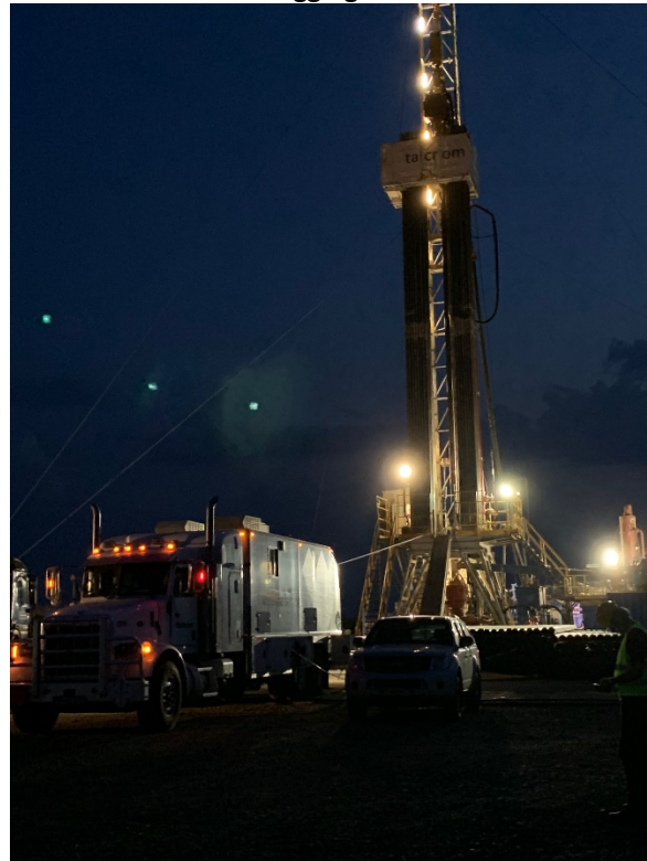
Electric line logging in 8 1/2" hole
