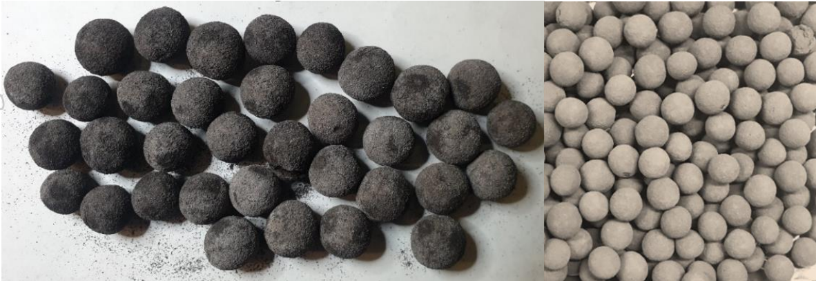
Figure 1: Vanadium rich iron concentrate pellets produced during bench-scale roast testing
