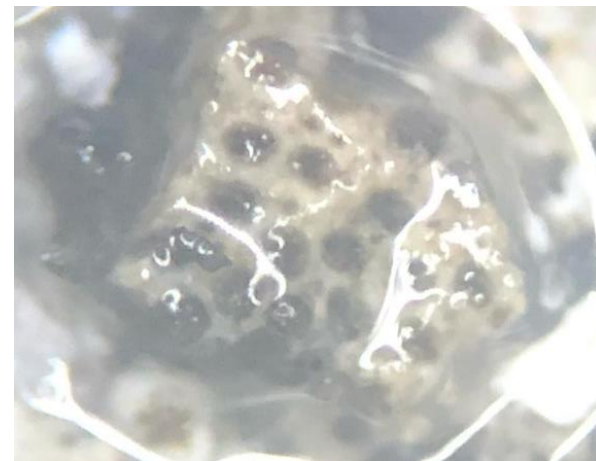
Above: Kingia reservoir showing visible porosity resultant from clay coated sand grains
